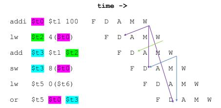
Without forwarding, the register values become available in the write-back phase, and are needed in the decode phase.
