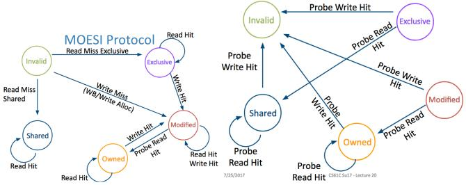
With the MOESI concurrency protocol implemented, accesses to cache accesses appear *serializiable*. This means that the result of the parallel cache accesses appear the same as if there were done in serial from one processor in some ordering.
