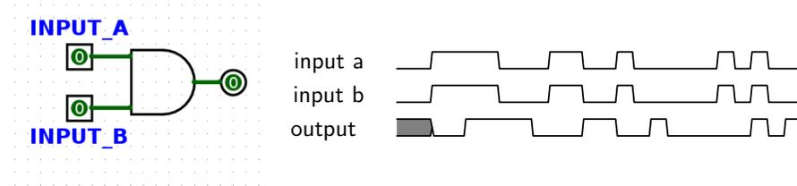
You should notice that the output of this AND gate always changes 2ps after its inputs change.
