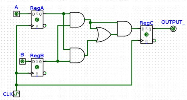
The maximum allowable hold time for RegC is how long it takes for RegC's input to change, so  $(\text{clk-to-q of A or B}) + \text{shortest CL time} = 4 + (5 + 5) = 14 \text{ ns}$ .
