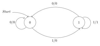
The FSM outputs a 1 if it detects the pattern "11". The FSM would output "001000000110"
