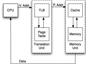
A chunk of memory or disk with a set size. Addresses in the same virtual page map to addresses in the same physical page. The page table determines the mapping.
