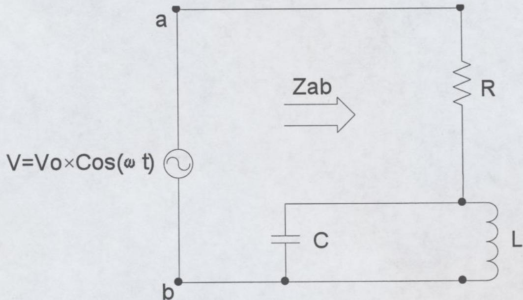
Find an expression for  $\omega$  (in terms of circuit variables  $L$ ,  $C$ , and/or  $R$ ) such that  $Z_{ab}$  (the impedance across nodes a and b) is purely resistive.
