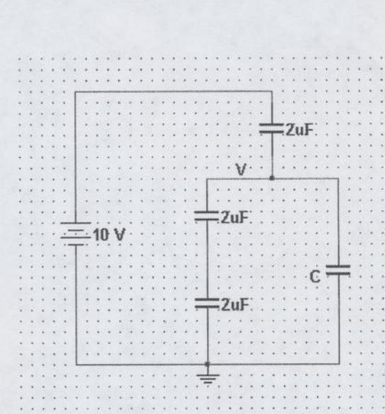
$$\begin{aligned} C_{eq} &= (\frac{1}{2\mu F} + \frac{1}{2\mu F})^{-1} + C \\ V &= 5V \\ 2\mu F &= C_{eq} \\ 2\mu F &= \frac{4(\mu F)}{4\mu F} + C \\ C &= 1\mu F \end{aligned}$$
