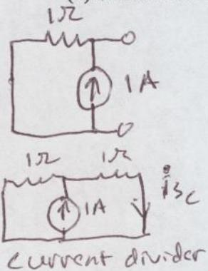
$$V_{oc} = (1A)(1\Omega) = 1V$$
