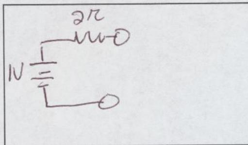
$$R_{Th} = \frac{V_{oc}}{i_{sc}} = 2\Omega$$
