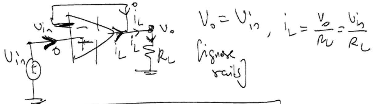
⇒  $V_{in}$  does not put out any current,
