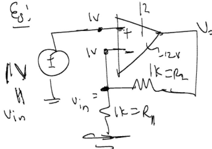
Non-inverting topology:  $V_o = \left(1 + \frac{R_f}{R_1}\right) V_{in}$
