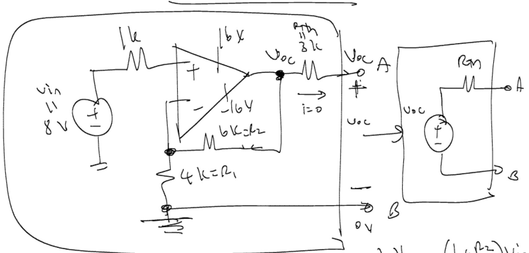
$V_{oc}$  = Output voltage of the op-amp
