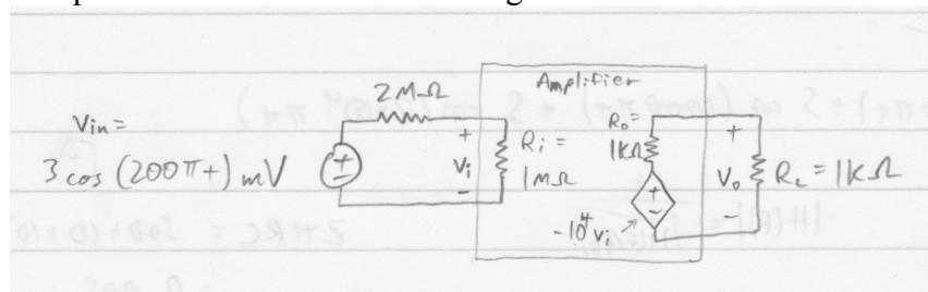
$$V_i = V_{in} \frac{1M\Omega}{1M\Omega + 2M\Omega} = 1 \cos(200\pi t) \text{ mV}$$
