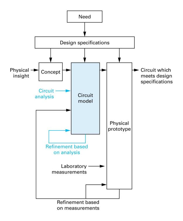
Figure 1.4 A conceptual model for electrical engineering design
