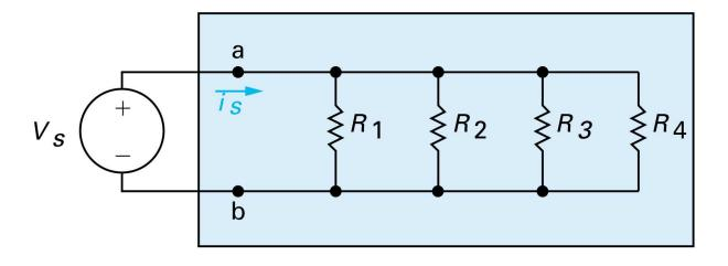
Figure 3.5 Resistors in parallel.
