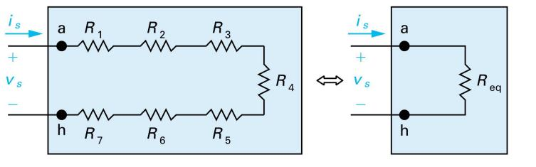
Figure 3.4 The black box equivalent of the circuit shown in Fig. 3.2.
