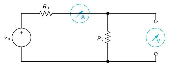
Figure 3.19 A short-circuit model for the ideal ammeter, and an open-circuit model for the ideal voltmeter.
