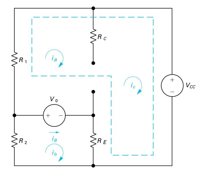
**Figure 4.28** The circuit shown in Fig. 4.27, depicting the supermesh created by the presence of the dependent current source.
