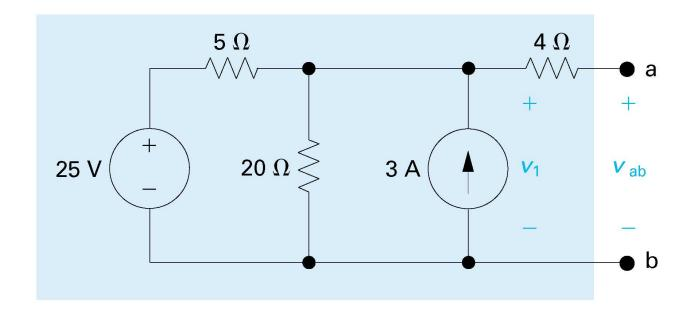
Figure 4.45 A circuit used to illustrate a Thevenin equivalent.
