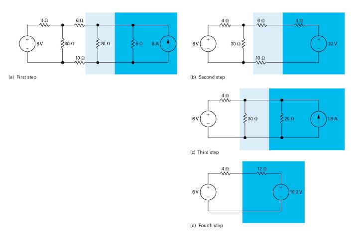
Figure 4.38 Step-by-step simplification of the circuit shown in Fig.4.37.
