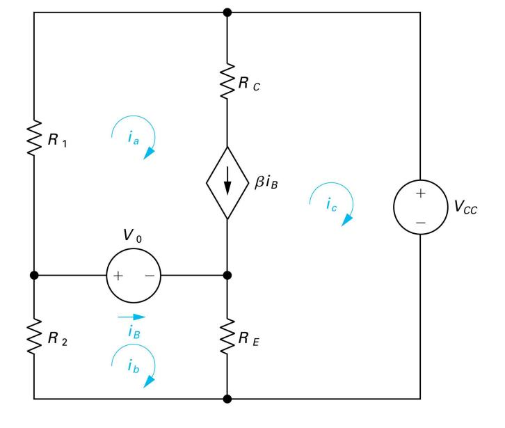
**Figure 4.27** The circuit shown in Fig. 2.24 with the mesh currents  $i_{\rm a}$ ,  $i_{\rm b}$ , and  $i_{\rm c}$ .
