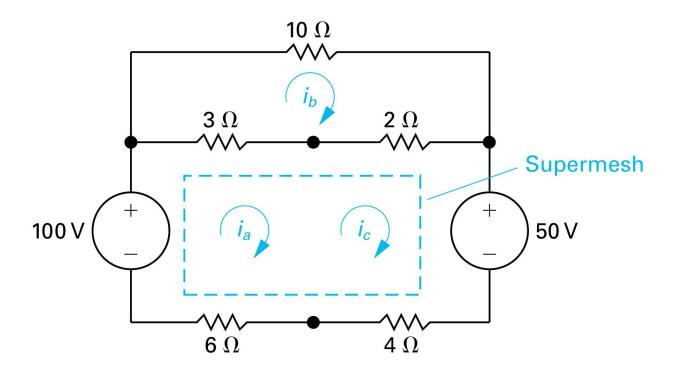
**Figure 4.26** The circuit shown in Fig. 4.25, illustrating concept of a supermesh.
