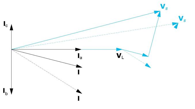
Figure 9.57 The effect of adding a load-shunting capacitor to the circuit shown in Fig. 9.53 if  ${\bf V}_{\rm L}$  is held constant.
