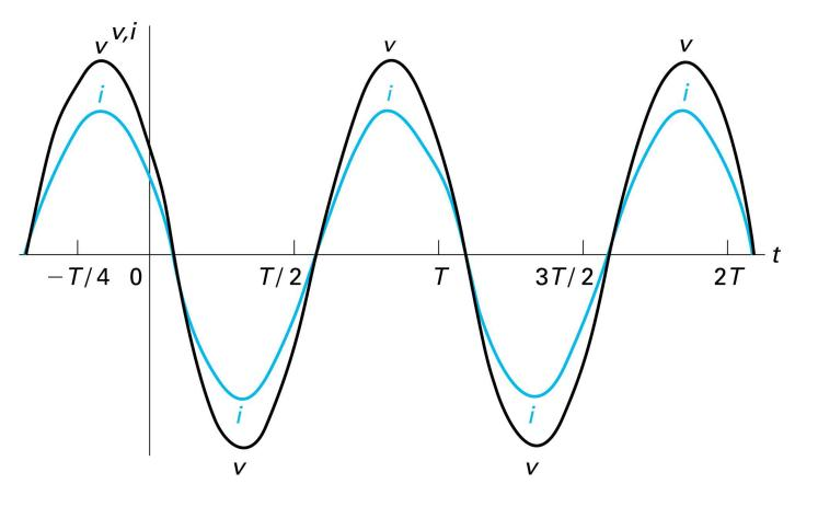
Figure 9.9 A plot showing that the voltage and current at the terminals of a resistor are in phase.
