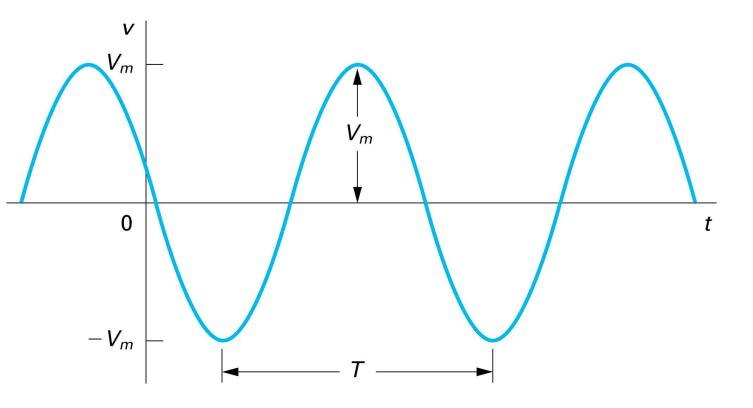
Figure 9.1 A sinusoidal voltage.
