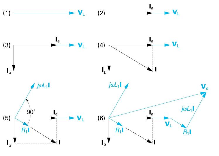
**Figure 9.54** The step-by-step evolution of the phasor diagram for the circuit in Fig. 9.53.
