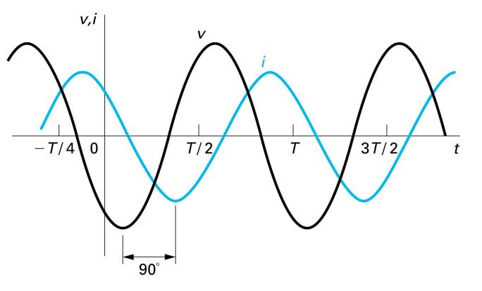
**Figure 9.11** A plot showing the phase relationship between the current and voltage at the terminals of an inductor ( $\theta_i = 60^\circ$ ).
