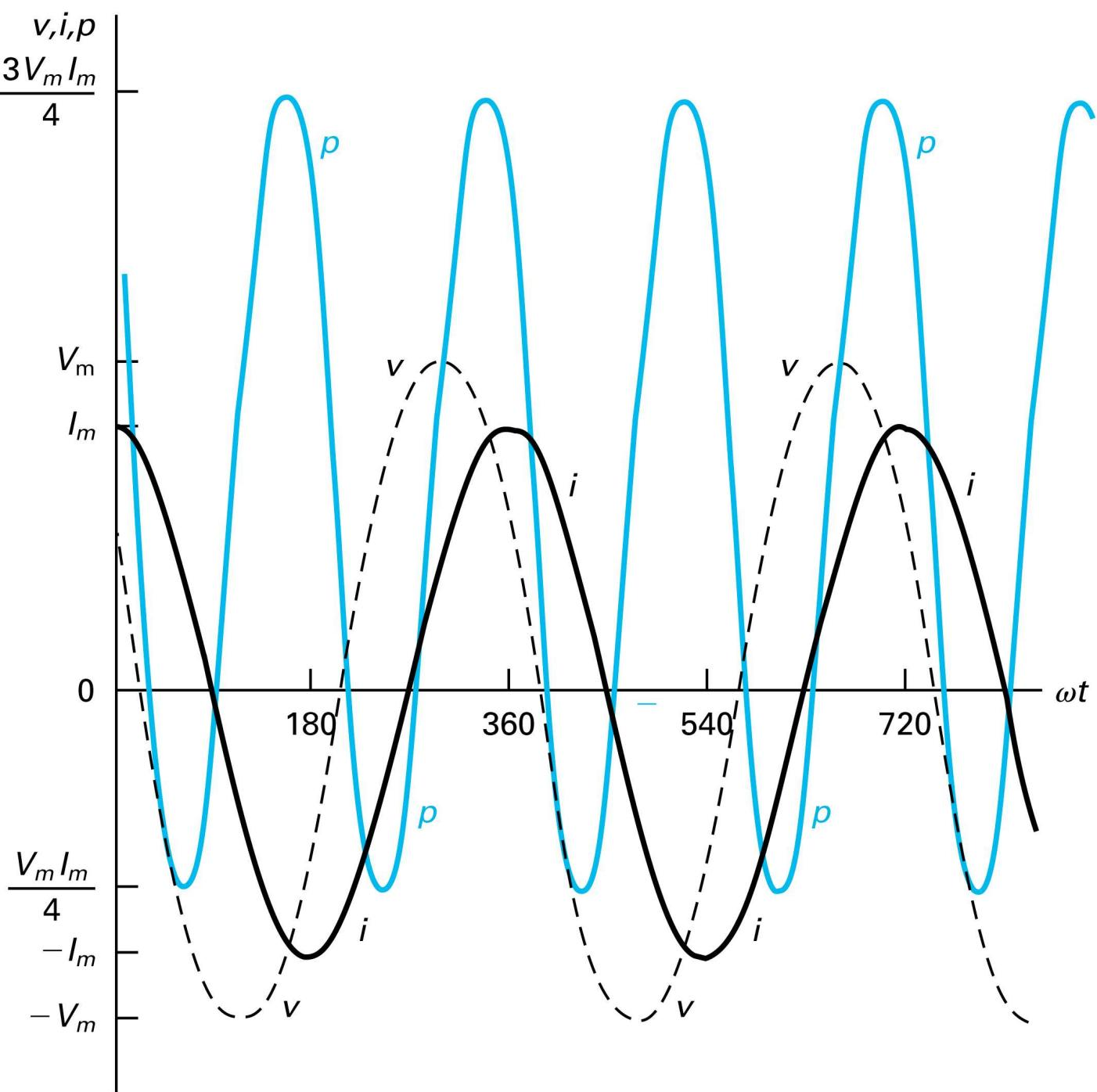
**Figure 10.2** Instantaneous power, voltage, and current versus  $\omega t$  for steady-state sinusoidal operation.
