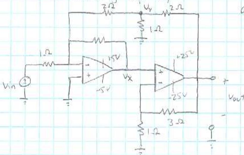
a.) Assume both op-amps are ideal & find  $V_{out}/V_{in}$
