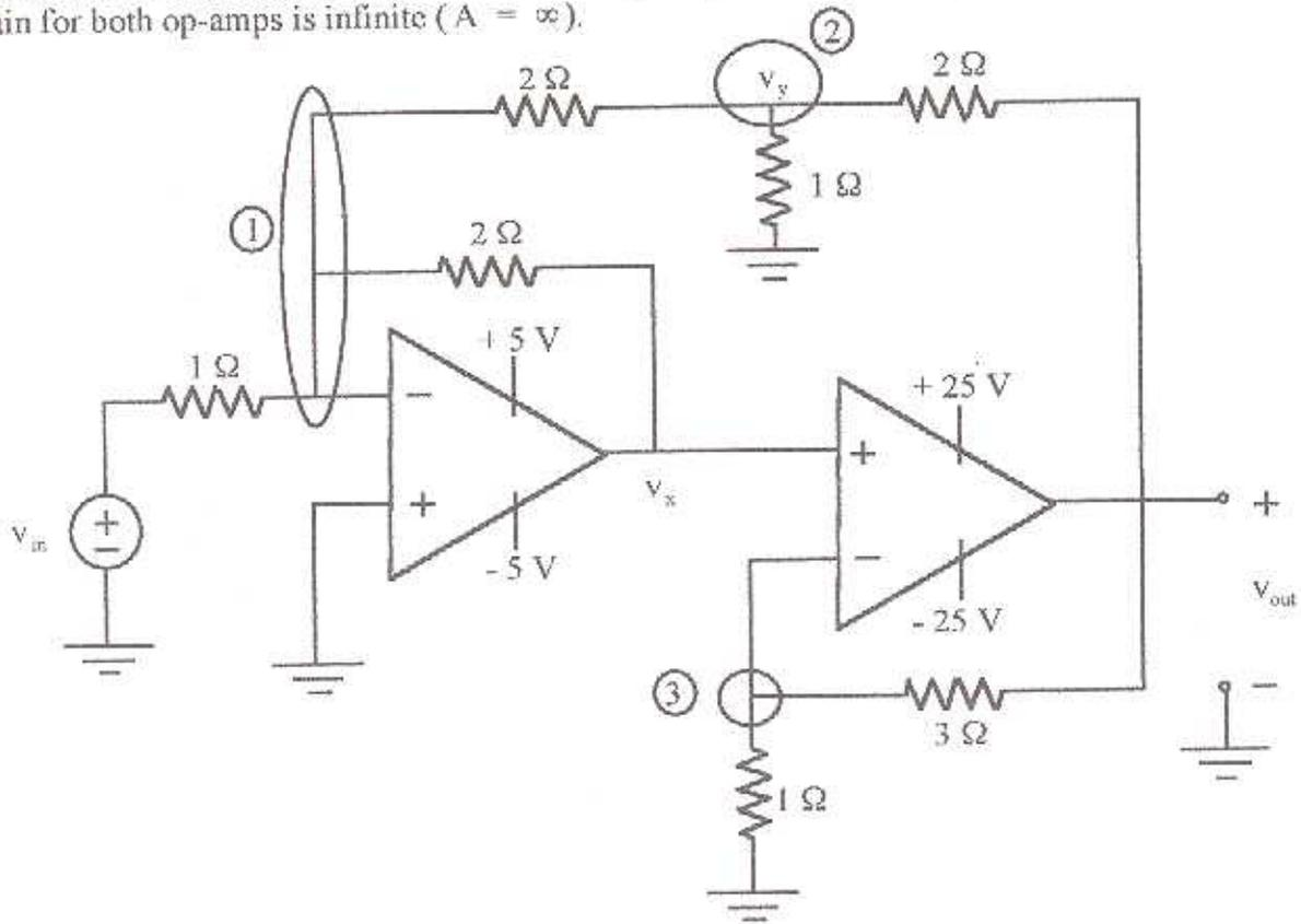
a.) Is the above circuit inverting or non-inverting? Answer this by inspection only. Explain your logic.
