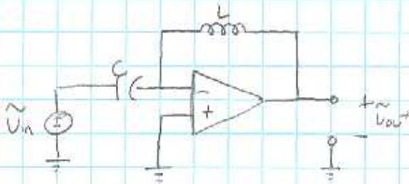
$$\begin{aligned} \tilde{V}_in &= \sin(\omega t) \\ \omega &= 1000 \text{ rad/sec} \\ L &= 1 \text{ mH} \\ C &= 1 \text{ mF} \end{aligned}$$
