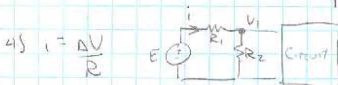
$i = \frac{E \cdot V_1}{R_1}$    NOT    $i = \frac{E}{R_1}$
