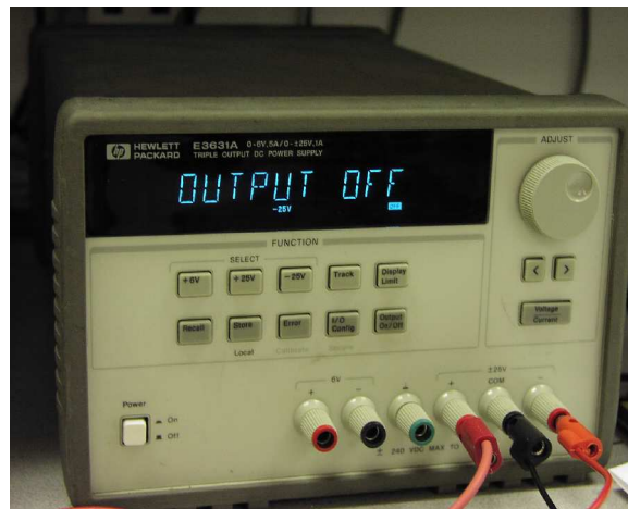
Figure 7. You need to turn the output on before you can set the power supply inputs
