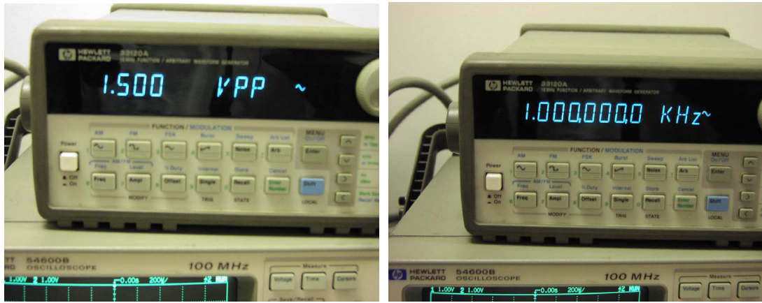
Figure 12. Function generator settings for parts i and ii.
