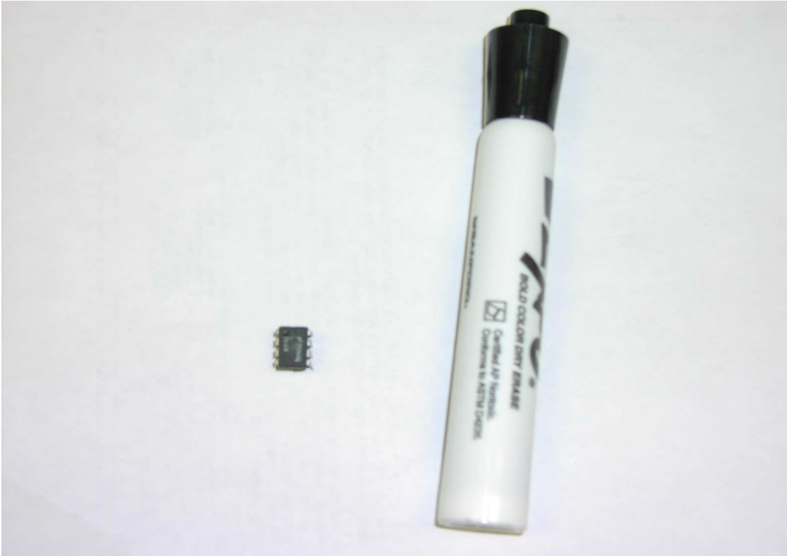
Figure 8. Comparing the op-amp IC to a whiteboard marker
