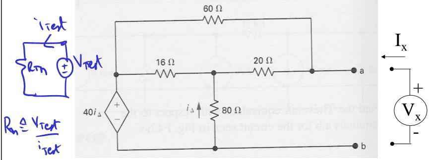
Since there is no independent source and we cannot arbitrarily turn off the dependence source, we can add a voltage source  $V_x$  across terminals a-b and measure the current through this terminal  $I_x$ .  $R_{th} = V_x / I_x$
