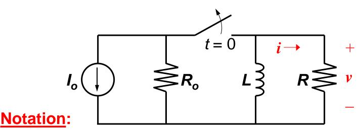
0<sup>-</sup> is used to denote the time just prior to switching0<sup>+</sup> is used to denote the time immediately after switching
