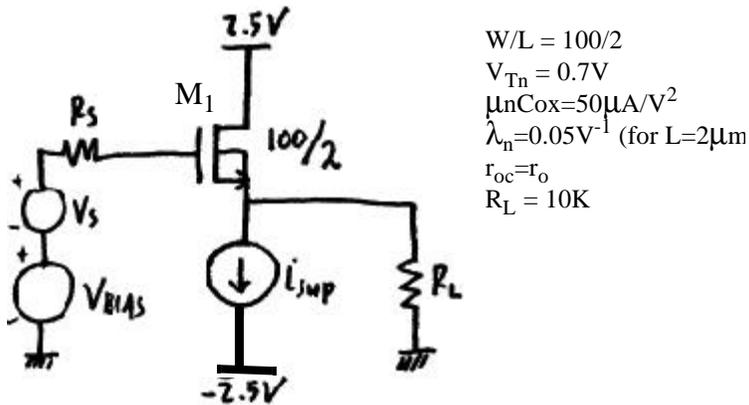
a) Assume  $V_{bs} = 0V$ , and find  $V_{bias}$  so that  $I_{sup} = 500 \mu A$ . (12pts)
