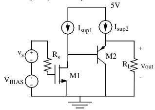
a) Draw the small signal model for this amplifier (Make sure to properly mark the g, s and d nodes for M1, and b, c, and e nodes for M2. Include  $r_{oc1}$ ,  $r_{oc2}$  due to  $I_{sup1}$  and  $I_{sup2}$ , respectively). (6 points)
