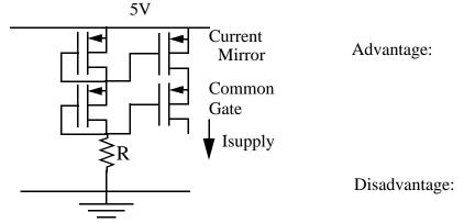
The following multistage amplifier is meant to deliver a voltage signal to a relatively small ohmic load of  $1K\Omega$ . Mark your choice of the last stage, and write a brief justification.
