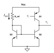
$$I_{REF} = \frac{V_{CC} - V_{BE3}}{R_{BEE}}$$
