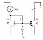
$$\begin{aligned} V_{GS} &= V_{TN} + \sqrt{\frac{2I_{REF}}{K_n \left(1 + \lambda V_{DS1}\right)}} \\ I_O &= I_{D2} = \frac{K_n}{2} \left(V_{GS} - V_{TN}\right)^2 \\ I_O &= I_{REF} \end{aligned}$$
