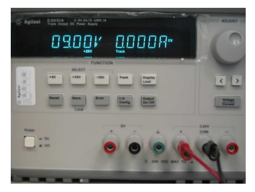
Figure 1: Agilent E3631A front panel.
