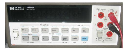
**Figure 1:** HP34401A front panel. The input cables on the right are set to measure voltage. To measure current, the red cable is moved to the bottom-right port while the connection for the black cable remains unchanged.
