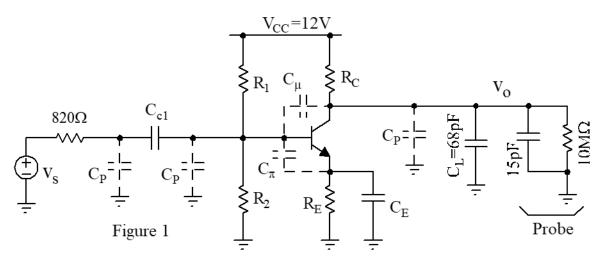
Note that there is no output coupling capacitor in Fig. 1. This lab has three phases: hand design, SPICE simulation, and lab verification. You must write a complete laboratory report describing your efforts in a professional-looking format, e.g., with figure captions, tables, etc.
