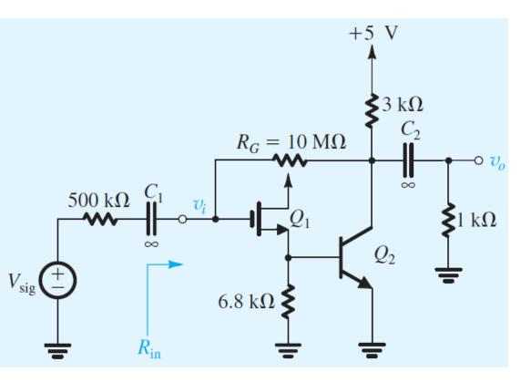
Unless otherwise specified, use  $\beta_F = 100$ ,  $V_A = 70$  V,  $K_p = K_n = 1 \text{ mA/V}^2$ ,  $V_{TN} = -V_{TP} = 1$  V, and  $\lambda = 0.02 \text{ V}^{-1}$ .
