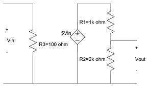
a) Find the open circuit voltage gain, Vout/Vin, of this amplifier.
