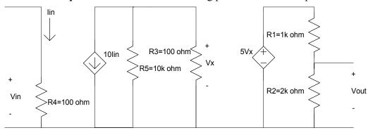
a) Draw the single standard two-port voltage amplifier that is equivalent to the above pair of amplifiers.
