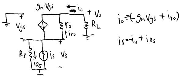
Since  $r_o \gg R_s$  ( $200\text{ k}\Omega$  vs.  $10\text{ k}\Omega$ ), neglect  $r_o$
