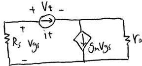
$$\begin{aligned} V_t &= -i_t \cdot R_s + (g_m V_{gs} - i_t) \cdot R_o \\ &= -i_t \cdot R_s - g_m \cdot R_o \cdot R_s \cdot i_t - i_t \cdot R_o \\ &= -i_t \cdot (R_s + R_o + g_m \cdot R_o \cdot R_s) \end{aligned}$$
