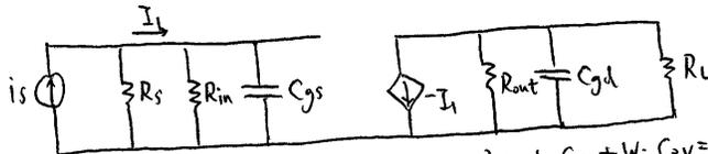
$$T_{Cgs} = (R_s \parallel R_{in}) \cdot C_{gs}$$
