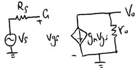
$$A_v = \frac{V_o}{V_s} = \frac{-g_m \cdot r_o \cdot V_{gs}}{V_s} = -\frac{g_m \cdot r_o \cdot V_s}{V_s} = -g_m \cdot r_o = \boxed{-89.4}$$
