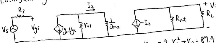
$$R_{out} = g_m R_{o2} \cdot R_{o1} + R_{o2}, \quad V_s = V_{gs}$$
