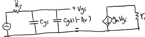
$$C_{gs} = \frac{2}{3} \cdot W \cdot L \cdot C_{ox} + W \cdot C_{ov} = \frac{2}{3} \cdot 40 \mu m \cdot 2 \mu m \cdot 2.3 \text{ fF} / \mu m^2 = 122.7 \text{ fF} + 20 \text{ fF} = 142.7 \text{ fF}$$
