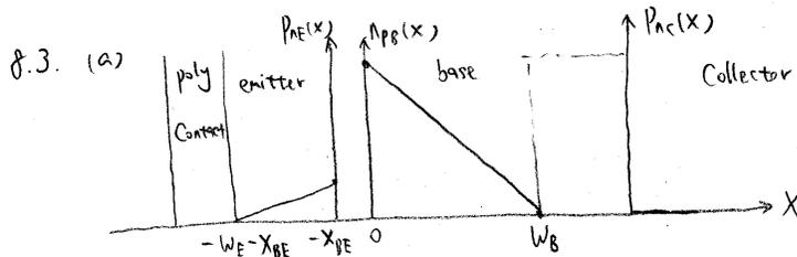
$$(b) \quad \beta_F = \frac{1}{1 + \left( \frac{D_p N_{aB} W_B}{D_n N_{dE} W_E} \right)} = \frac{1}{1 + \left( \frac{5 \times 10^{17} \times 0.5 \times 10^{-4}}{5 \times 8 \times 10^{18} \times 10^{-4}} \right)} = \boxed{0.9938}$$
