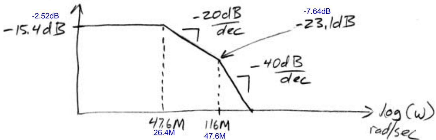
$$-15.4 - 20 \log\left(\frac{116}{47.6}\right) = -23.1 \text{ dB} \quad -2.52 - 20 \log(47.6/26.4) = -7.64 \text{ dB}$$
