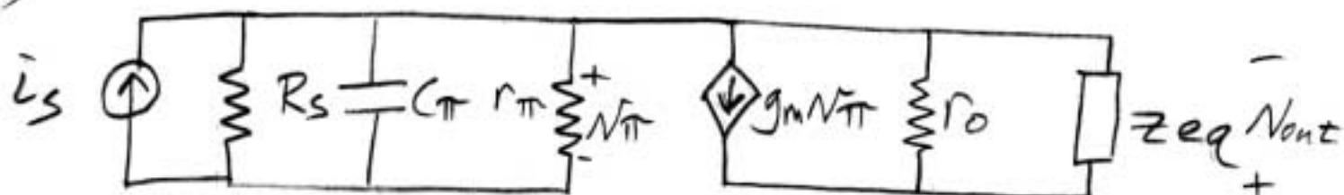
$$g_m = \frac{I_C}{V_{th}} = \frac{3 \times 10^{-3}}{26 \times 10^{-3}} = 0.115 A/V$$
