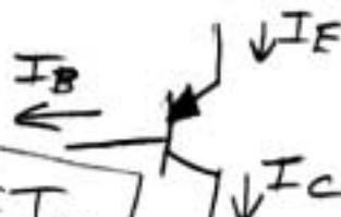
$$I_C = \frac{V_{out}}{Z_{eq}(w=0)} = \frac{2.5}{833} = 3mA = I_C$$
