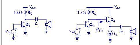
Since the emitter follower increases the load resistance to a much higher value, it is suited as a buffer between a CE stage and a heavy load resistance to alleviate the problem of gain degradation.
