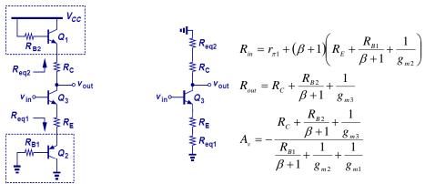
Impedances seen at the emitter of Q<sub>1</sub> and Q<sub>2</sub> can be lumped with R<sub>C</sub> and R<sub>E</sub>, respectively, to form the equivalent emitter and collector impedances.
