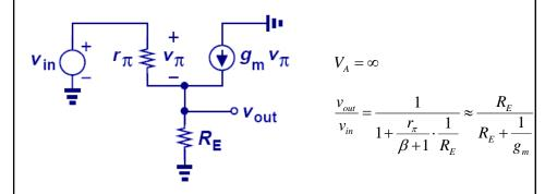
As shown above, the voltage gain is less than unity and positive.
