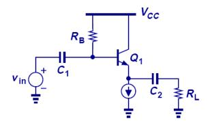
By putting a constant current source at the emitter, the bias current, V<sub>BE</sub>, and I<sub>B</sub>R<sub>B</sub> are fixed regardless of the supply value.
