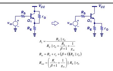
Since r<sub>O</sub> is in parallel with R<sub>E</sub>, its effect can be easily incorporated into voltage gain and input and output impedance equations.
