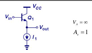
The voltage gain is unity because a constant collector current (= I<sub>1</sub>) results in a constant V<sub>BE</sub>, and hence Vout follows Vin exactly.
