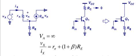
The input impedance of emitter follower is exactly the same as that of CE stage with emitter degeneration. This is not surprising because the input impedance of CE with emitter degeneration does not depend on the collector resistance.
