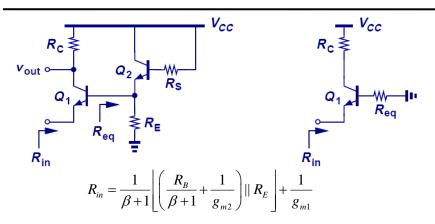
The key for solving this problem is recognizing the equivalent base resistance of  $\mathbf{Q}_1$  is the parallel connection of RE and the impedance seen at the emitter of Q<sub>2</sub>.
