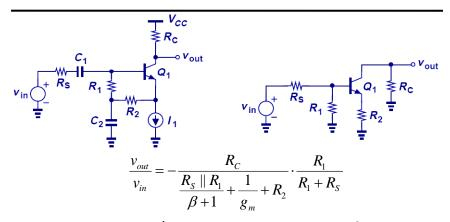
Again, AC ground/short and Thevenin transformation are needed to transform the complex circuit into a simple stage with emitter degeneration.
