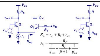
The key for solving this problem is first identifying R<sub>eq</sub>, which is the impedance seen at the emitter of Q<sub>2</sub> in parallel with the infinite output impedance of an ideal current source. Second, use the equations for degenerated CE stage with RE replaced by R<sub>eq</sub>.
