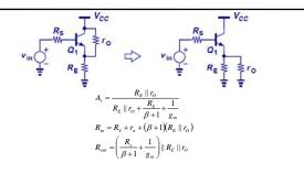
Since r<sub>O</sub> is in parallel with R<sub>E</sub>, its effect can be easily incorporated into voltage gain and input and output impedance equations.
