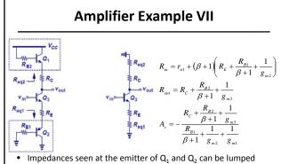
with  $R_C$  and  $R_E$ , respectively, to form the equivalent emitter and collector impedances.
