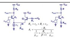
$\bullet~$  The key for solving this problem is first identifying  $R_{\rm eq},$  which is the impedance seen at the emitter of Q<sub>2</sub> in parallel with the infinite output impedance of an ideal current source. Second, use the equations for degenerated CE stage with RE replaced by  $R_{\rm eq}$ .
