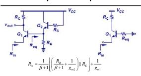
• The key for solving this problem is recognizing the equivalent base resistance of  $\mathbf{Q}_1$  is the parallel connection of RE and the impedance seen at the emitter of Q<sub>2</sub>.
