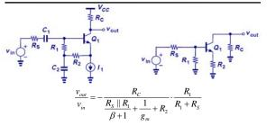
• Again, AC ground/short and Thevenin transformation are needed to transform the complex circuit into a simple stage with emitter degeneration.
