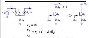
• The input impedance of emitter follower is exactly the same as that of CE stage with emitter degeneration. This is not surprising because the input impedance of CE with emitter degeneration does not depend on the collector resistance.
