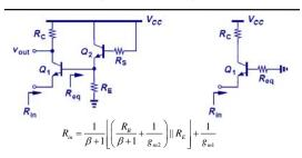
• The key for solving this problem is recognizing the equivalent base resistance of  $\mathbf{Q}_{\mathbf{1}}$  is the parallel connection of RE and the impedance seen at the emitter of Q<sub>2</sub>.
