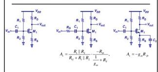
Degeneration is used to stabilize bias point, and a bypass capacitor can be used to obtain a larger small-signal voltage gain at the frequency of interest.
