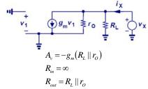
• However, channel length modulation leads to finite output resistance,  $r_{o}$ , which is in parallel with the load resistance, R<sub>L</sub>
