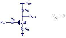
Since at low frequencies, the gate conducts no current, gate resistance does not affect the gain or I/O impedances.
