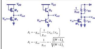
• Lower gain, but less dependent on process parameters.
