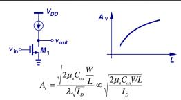
• Since  $\lambda$  is inversely proportional to L, the intrinsic voltage gain actually becomes proportional to the square root of L. EE105 Spring 2008
