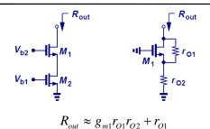
• In this example, the impedance that degenerates the CS stage is  $r_0$ , instead of  $1/g_m$  in the previous example.
