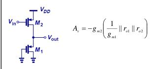
• Note that PMOS circuit symbol is usually drawn with the source on top of the drain.
