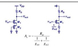
• A diode-connected device degenerates a CS stage.
