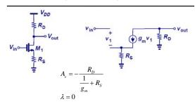
• Similar to bipolar counterpart, when a CS stage is degenerated, its gain, I/O impedances, and linearity change.
