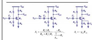
Degeneration is used to stabilize bias point, and a bypass capacitor can be used to obtain a larger small-signal voltage gain at the frequency of interest.
