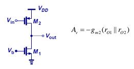
• Similarly, with PMOS as input stage and NMOS as the load, the voltage gain is the same as before.
