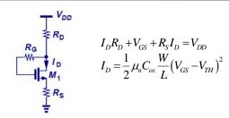
The circuit above is analyzed by noting M<sub>1</sub> is in saturation and no potential drop appears across RG.
