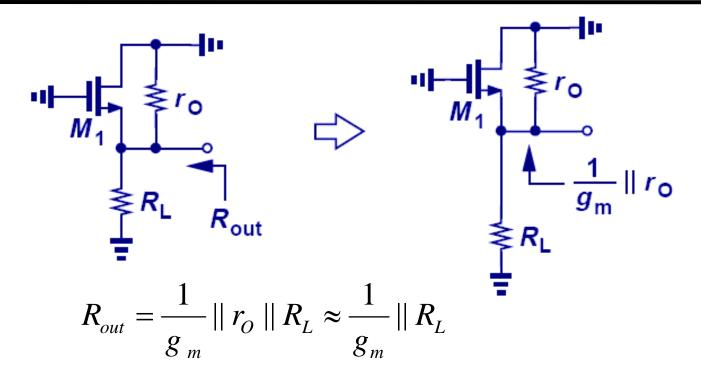
• The output impedance of a source follower is relatively low, whereas the input impedance is infinite (at low frequencies); thus, a good candidate as a buffer.
