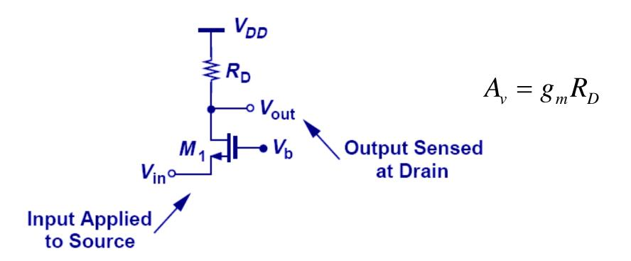
Common-gate stage is similar to common-base stage: a rise in input causes a rise in output. So the gain is positive.
