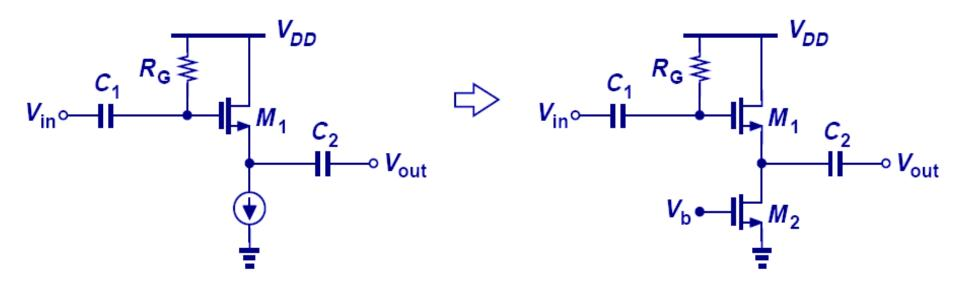
If R<sub>s</sub> is replaced by a current source, drain current I<sub>D</sub> becomes independent of supply voltage.
