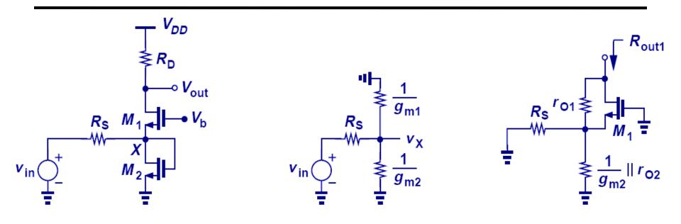
$$\frac{v_{out}}{v_{in}} = \frac{g_{m1}R_D}{1 + (g_{m1} + g_{m2})R_S}$$
