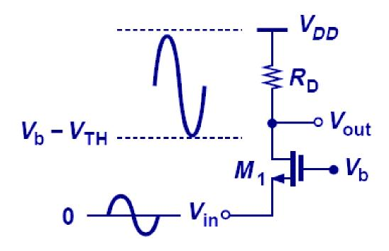
• In order to maintain M1 in saturation, the signal swing at  $V_{out}$  cannot fall below  $V_b-V_{TH}$
