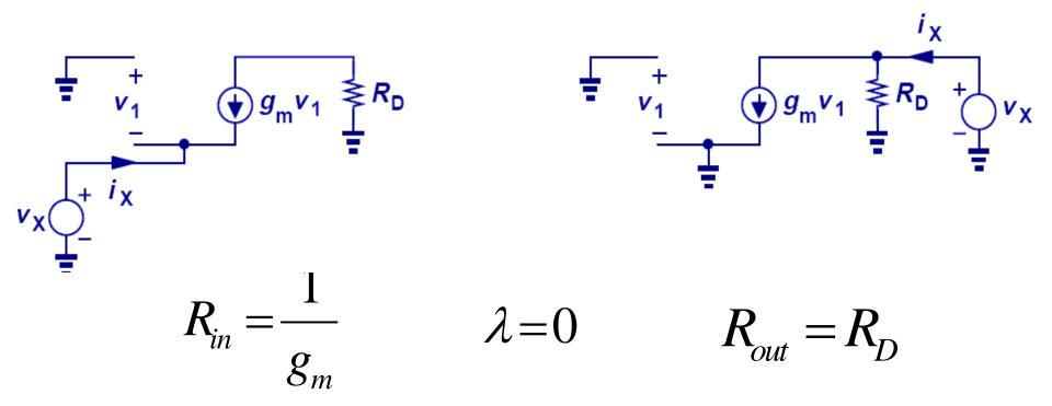
• The input and output impedances of CG stage are similar to those of CB stage.
