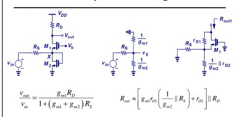
Diode-connected M2 acts as a resistor to provide the bias current.
