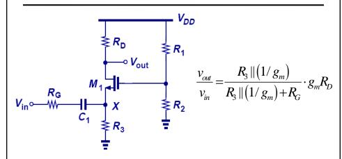
R<sub>1</sub> and R<sub>2</sub> provide gate bias voltage, and R<sub>3</sub> provides a path for DC bias current of M<sub>1</sub> to flow to ground.
