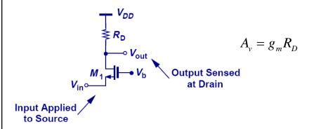
Common-gate stage is similar to common-base stage: a rise in input causes a rise in output. So the gain is positive.
