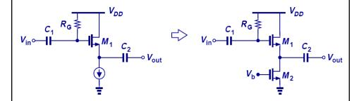
If R<sub>s</sub> is replaced by a current source, drain current I<sub>D</sub> becomes independent of supply voltage.
