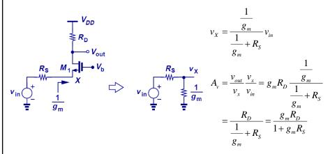
When a source resistance is present, the voltage gain is equal to that of a CS stage with degeneration, only positive.
