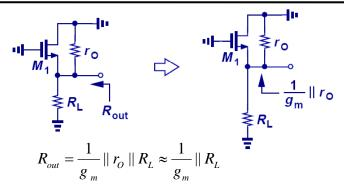
The output impedance of a source follower is relatively low, whereas the input impedance is infinite (at low frequencies); thus, a good candidate as a buffer.
