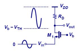
In order to maintain M1 in saturation, the signal swing at V<sub>out</sub> cannot fall below V<sub>b</sub>-V<sub>TH</sub>
