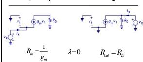
• The input and output impedances of CG stage are similar to those of CB stage.
