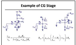
• Diode-connected M2 acts as a resistor to provide the bias current.
