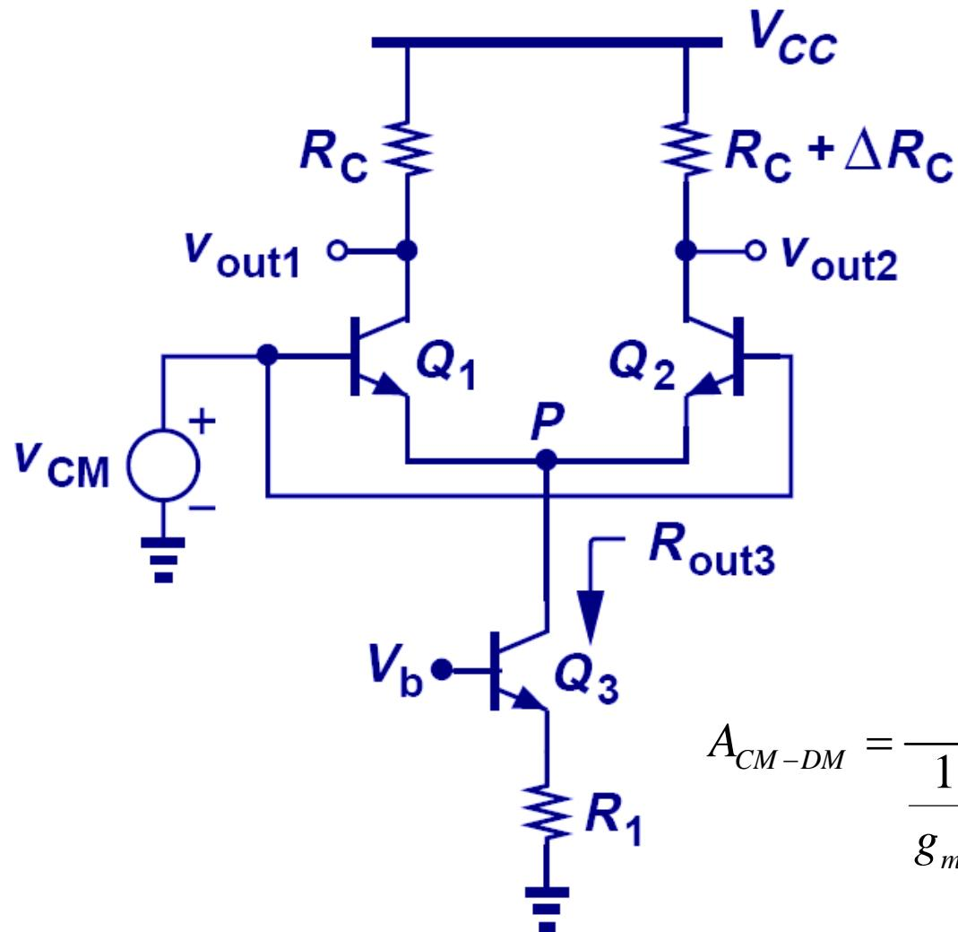
$$A_{CM-DM} = \frac{\Delta R_C}{\frac{1}{g_{m1}} + 2 \{ [1 + g_{m3}(R_1 \parallel r_{\pi 3})]r_{O3} + R_1 \parallel r_{\pi 3} \}}$$
