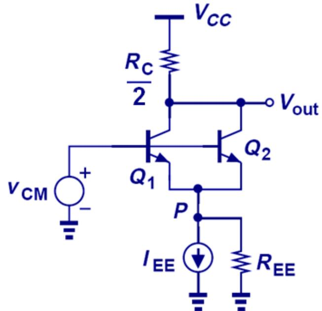
$$\frac{\Delta V_{out,CM}}{\Delta V_{in,CM}} = -\frac{(R_C/2)}{\frac{1}{2g_m} + R_{EE}} = -\frac{R_C}{\frac{1}{g_m} + 2R_{EE}}$$
