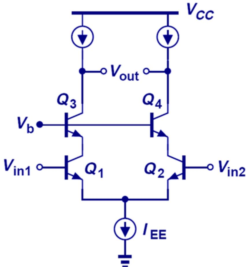
$$R_{out} = [1 + g_{m3}(r_{O1} \parallel r_{\pi3})]r_{O3} + r_{O1} \parallel r_{\pi3}$$
