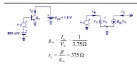
Here, small signal parameters are calculated from DC operating point and are used to calculate the change in collector current due to a change in V<sub>BE</sub>.
