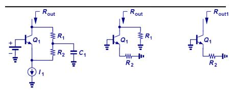
$$R_{out} = R_1 \parallel R_{out1} \longrightarrow R_{out1} = \left[1 + g_m(R_2 \parallel r_\pi)\right] r_o \longrightarrow R_{out} = \left[1 + g_m(R_2 \parallel r_\pi)\right] r_o \parallel R_1$$
