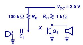
Since the speaker has an inductor, connecting it directly to the amplifier would short the collector at DC and therefore push the transistor into deep saturation.
