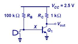
Since the microphone has a very low resistance that connects from the base of Q<sub>1</sub> to ground, it attenuates the base voltage and renders Q<sub>1</sub> without a bias current.
