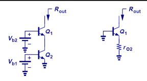
$$R_{out} = [1 + g_{m1}(r_{O2} || r_{\pi 1})] r_{O1}$$
