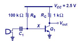
Capacitor isolates the bias network from the microphone at DC but shorts the microphone to the amplifier at higher frequencies.
