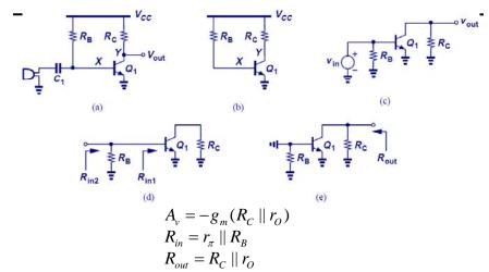
Coupling capacitor is open for DC calculations and shorted for AC calculations.
