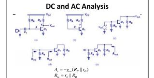
$R_{out} = R_C \parallel r_O$ • Coupling capacitor is open for DC calculations and shorted for AC calculations.
