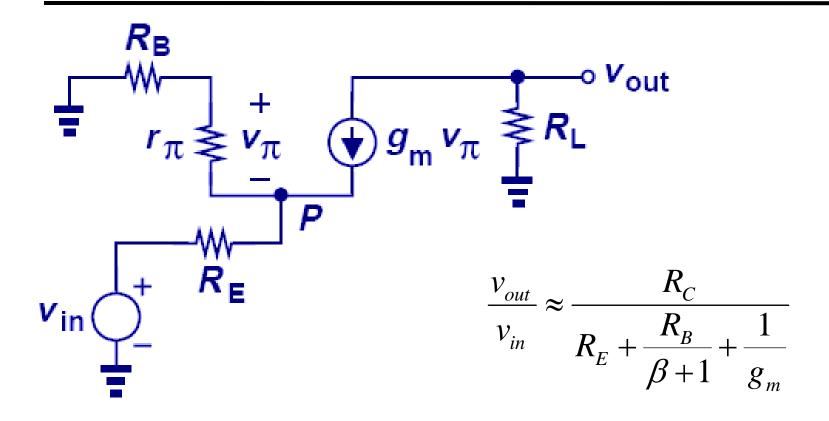
With an addition of base resistance, the voltage gain degrades.
