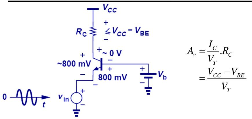
• To maintain the transistor out of saturation, the maximum voltage drop across  $R_{\rm C}$  cannot exceed  $V_{\rm CC}$ -  $V_{\rm BE}$ .
