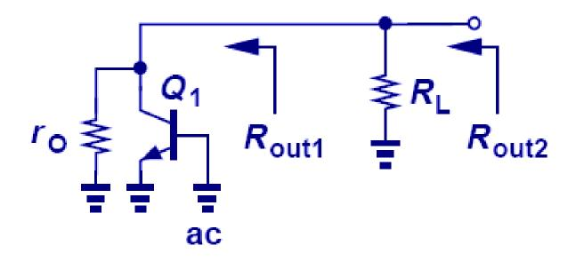
$$R_{out} = r_O \parallel R_L$$
