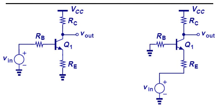
The voltage gain of CB amplifier with base resistance is exactly the same as that of CE stage with base resistance and emitter degeneration, except for a negative sign.
