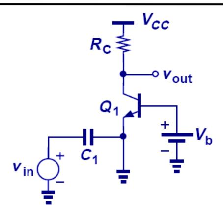
The input signal is shorted to ground. The circuit still does not amplify.
