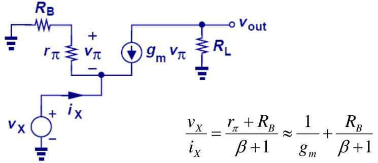
• The input impedance of CB with base resistance is equal to  $1/g_m$  plus  $R_B$  divided by ( $\beta$ +1). This is in contrast to degenerated CE stage, in which the resistance in series with the emitter is multiplied by ( $\beta$ +1) when seen from the base.
