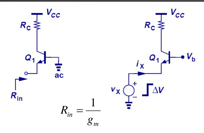
The input impedance of CB stage is much smaller than that of the CE stage.
