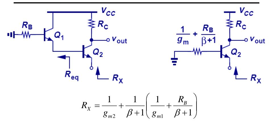
• To find the  $R_X$ , we have to first find  $R_{eq}$ , treat it as the base resistance of  $Q_2$  and divide it by  $(\beta+1)$ .
