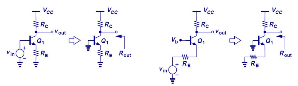
The output impedances of CE, CB stages are the same if both circuits are under the same condition. This is because when calculating output impedance, the input port is grounded, which renders the same circuit for both CE and CB stages.
