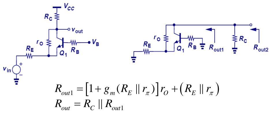
The output impedance of CB stage is equal to R<sub>c</sub> in parallel with the impedance looking down into the collector.
