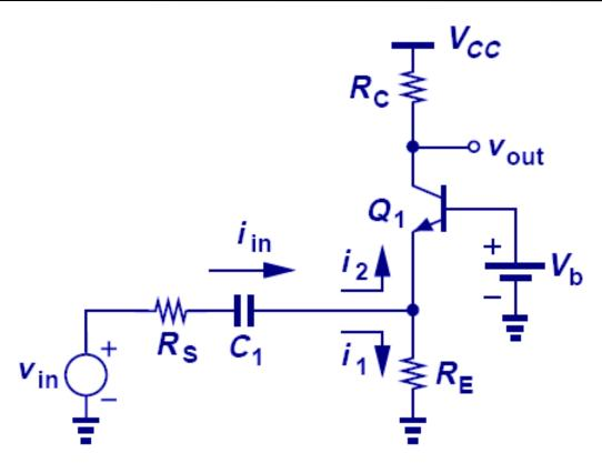
• The reduction of input impedance due to  $R_E$  is bad because it shunts part of the input current to ground instead of to  $Q_1$  (and  $R_C$ ).
