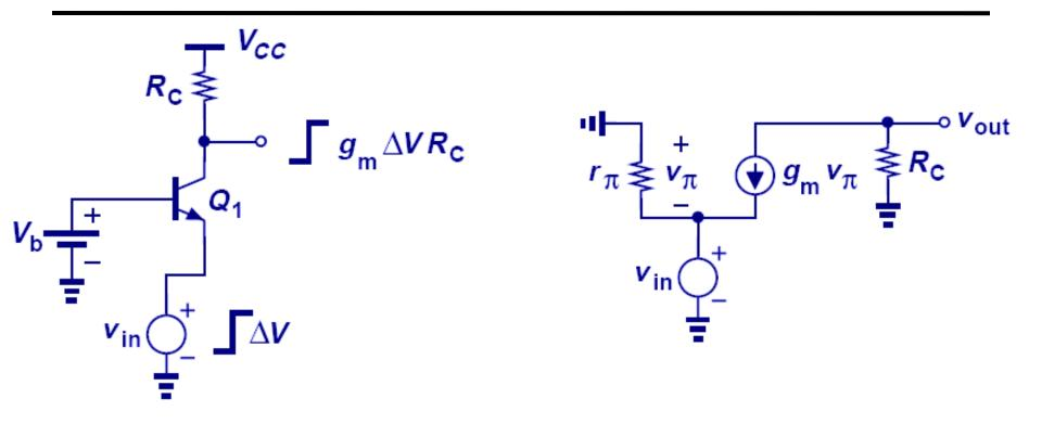
The voltage gain of CB stage is g<sub>m</sub>R<sub>C</sub>, which is identical to that of CE stage in magnitude and opposite in phase.
