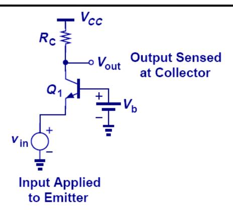
In common base topology, where the base terminal is biased with a fixed voltage, emitter is fed with a signal, and collector is the output.
