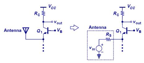
An antenna usually has low output impedance; therefore, a correspondingly low input impedance is required for the following stage.
