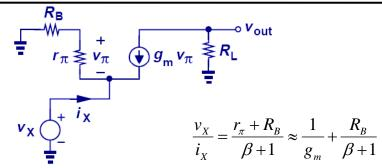
• The input impedance of CB with base resistance is equal to  $1/g_m$  plus  $R_B$  divided by  $(\beta+1)$ . This is in contrast to degenerated CE stage, in which the resistance in series with the emitter is multiplied by  $(\beta+1)$  when seen from the base.
