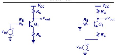
The voltage gain of CB amplifier with base resistance is exactly the same as that of CE stage with base resistance and emitter degeneration, except for a negative sign.
