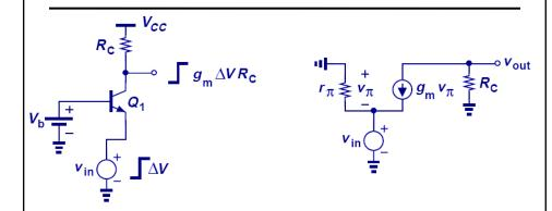
• The voltage gain of CB stage is  $g_m R_C$ , which is identical to that of CE stage in magnitude and opposite in phase.
