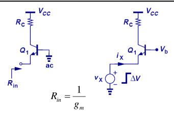
• The input impedance of CB stage is much smaller than that of the CE stage.
