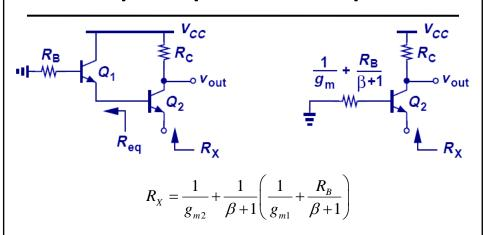
To find the R<sub>X</sub>, we have to first find R<sub>eq</sub>, treat it as the base resistance of Q<sub>2</sub> and divide it by (β+1).
