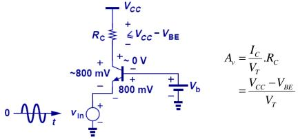
To maintain the transistor out of saturation, the maximum voltage drop across R<sub>C</sub> cannot exceed V<sub>CC</sub>-V<sub>BE</sub>.
