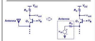
• An antenna usually has low output impedance; therefore, a correspondingly low input impedance is required for the following stage.
