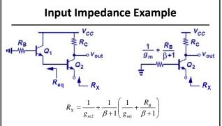
• To find the  $R_{\chi}$ , we have to first find  $R_{eq}$ , treat it as the base resistance of  $Q_2$  and divide it by ( $\beta$ +1).
