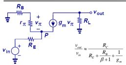
With an addition of base resistance, the voltage gain degrades.
