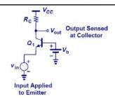
In common base topology, where the base terminal is biased with a fixed voltage, emitter is fed with a signal, and collector is the output.
