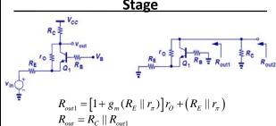
• The output impedance of CB stage is equal to R<sub>C</sub> in parallel with the impedance looking down into the collector.
