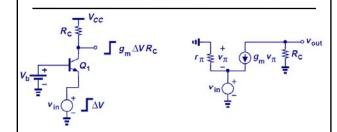
The voltage gain of CB stage is g<sub>m</sub>R<sub>C</sub>, which is identical to that of CE stage in magnitude and opposite in phase.
