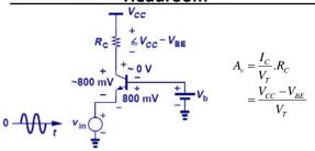
• To maintain the transistor out of saturation, the maximum voltage drop across  $\rm R_{\rm C}$  cannot exceed  $\rm V_{\rm CC}{}^{\rm -}$   $\rm V_{\rm BE}.$
