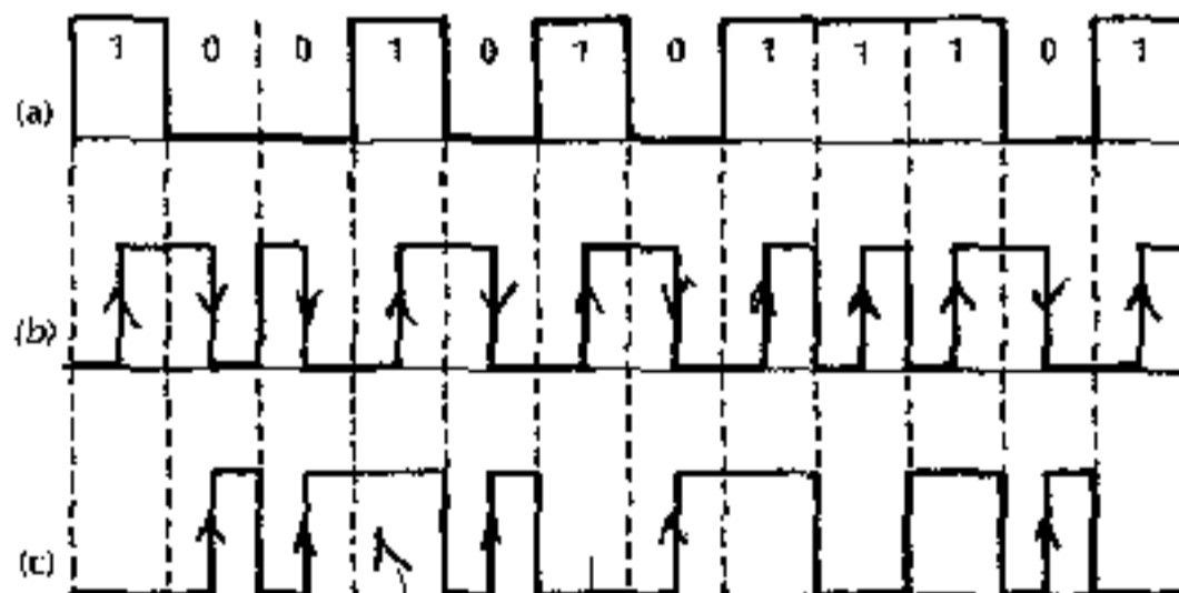
Figure 11.39 Examples of binary 1B2B codes used in optical fiber communications: (a) unencoded NRZ data; (b) biphase or Manchester encoding; (c) coded mark inversion (CMI) encoding.
