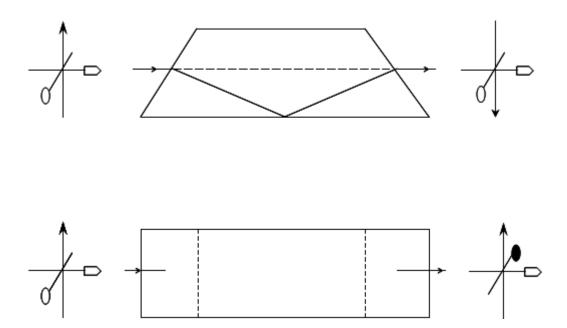
We see that the orientation of the lower image, compared to that of the upper image, is rotated around by  $180^{\circ}$ the longitudinal axis of the prism, while the lower prism is rotated only by  $90^{\circ}$  around its axis in the same direction.
