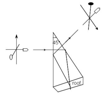
Yes, it can be used as an erecting prism!
