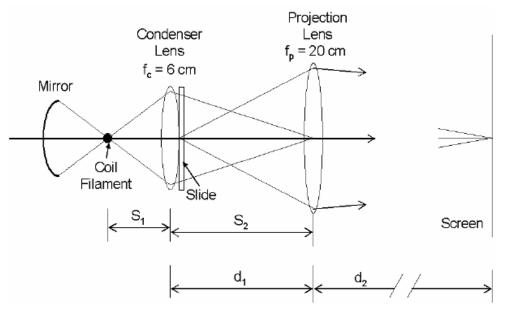
(b) The distance between the slide and the projector lens is  $s_2$  in the diagram.
