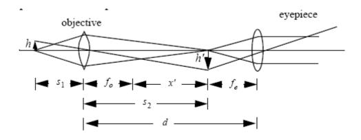
The eye can resolve an object size of  $\sim 0.08$ mm = 80 µm at the distance of 25 cm. To have a resolution of 1µm, the total magnification of the microscope is
