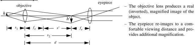
The total magnification is the product of the linear objective magnification times the eyepiece angular magnification.
