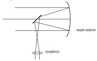
All modern astronomical telescopes have this basic configuration because it is much more practical to fabricate large mirrors than lenses. The size of the large main mirror (the entrance pupil) sets the diffraction limit. Also, a larger entrance pupil gathers more light, so that faint objects can be detected. Ground-based telescopes are limited by atmospheric turbulence, which introduces unavoidable aberrations. One solution is to go into space, above the atmosphere.
