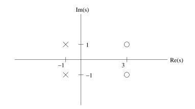
Since H(s) has exactly 2 zeros at infinity, H(s) has at least two more unknown finite poles. If H(s) has more than 4 poles, then it will have a zero at some finite location for every additional pole. Furthermore, because h(t) is causal and stable, all poles of H(s) must lie in the left half of the s-plane and the ROC must contain the  $j\omega$  axis.
