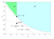
Optimizing over the slope  $-\lambda < 0$  of the line we can close the duality gap  $p^* - g(\lambda)$ .
